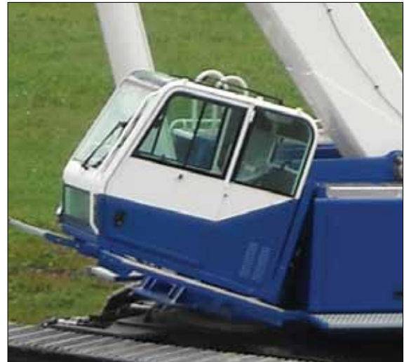
Standard operators cab tilts up for improved operator comfort. Improved design walkways allow easy access into the cab.
